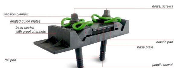
Figure 9: Structure of the rail fastening system DFF304 by Vossloh
